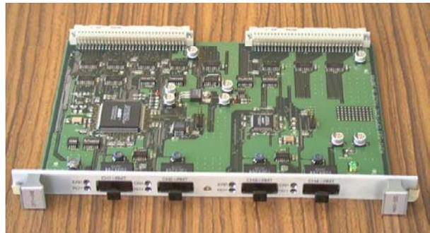
Figure 1: A view of new remote I/O master card.
