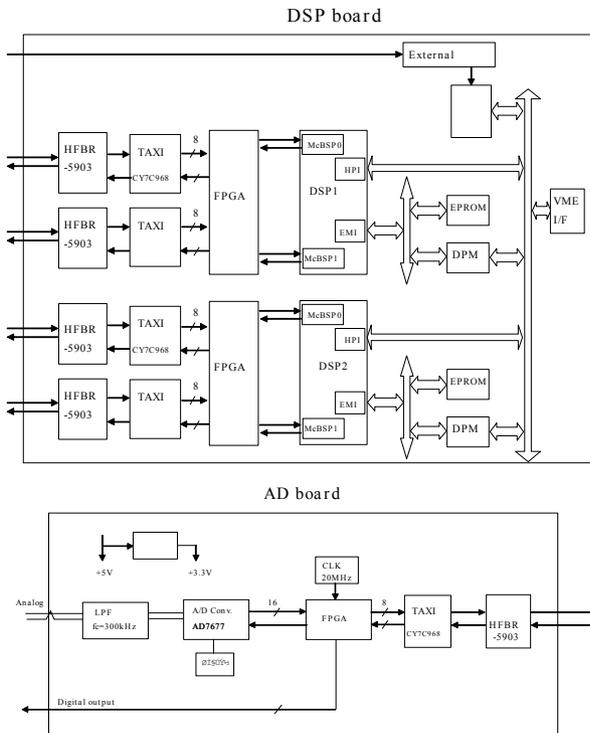
Figure 4: A block diagram of the DSP board and AD board.
