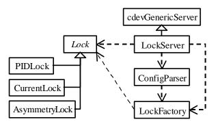
Figure 1: Simplified Lock Server Class Diagram
