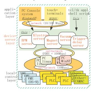
Figure 1: Simplified view of the control system.
