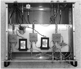
Figure 2. RF chassis for two Klystrons
