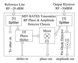
Figure 1. RF Detection Hardware architecture
