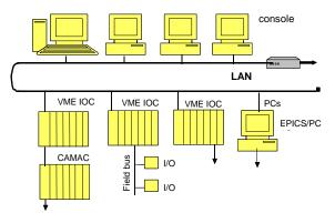
Figure 1: System architecture
