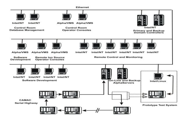
Figure 1: ATLAS Control System Showing Prototype Distributed I/O
