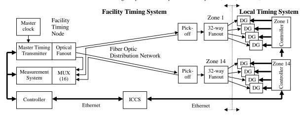
**Figure 1.** Block diagram showing major functional components of the NIF Integrated Timing System. MUX (multiplexer), DG (8-channel Delay Generator module).
