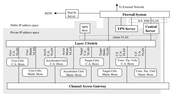
Figure 1: ICS Control System Network
