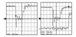
Fig.3. Examples of normal(left) and abnormal(right) DTACK\* signals.
