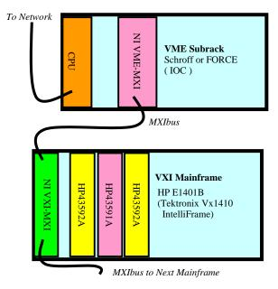
NI: National Instruments HP: Hewlett-Packard(Present Agilent Technology) HP43591A: FFT Module HP43592A: Multiplexer Module
