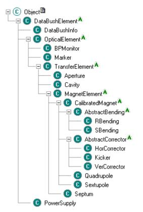
Figure 1: Diagram of element inheritance. All DataBush elements have one common ancestor, the DataBushElement.
