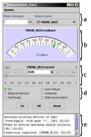
Figure2: Power Supply Panel. This panel was created from Abeans and GUI components in Java visual builder environment without typing a single line of code. The following GUI components can be seen: a) selector, b) gauger, c) slider, d) ledder, e) ATextPane a pane with messages for the user.
