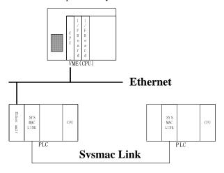
Fig. 1: PLC Wrapper system configuration.
