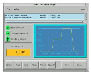
Figure 6: X-Windows Power Supply Control Interface
