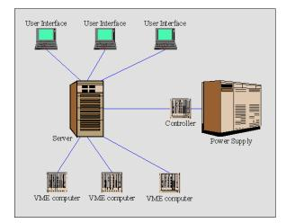
Figure 1: Architecture of the Power Control System
