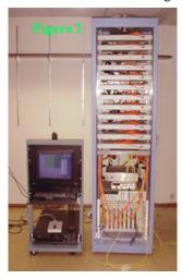
an IOC with 8 PSCs with 24 PSIs connected to four of the PSCs. The PSCs are using external triggers to read and write to the PSIs. The trigger rate is set at 4000Hz in this example to test operation under high load. For each PSI, the output voltage is fed back to the input connectors the and output commands are fed back to the status input to simulate a power supply.
