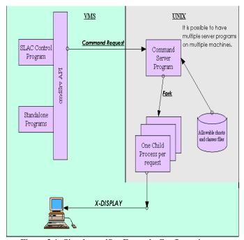
Figure 2.1: Simple cmdSrv Example Configuration
