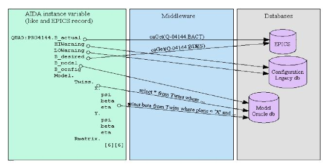
Figure 1: Logical Quadrupole device consists of data from different sources but accessible to the application via a single named hierarchy
