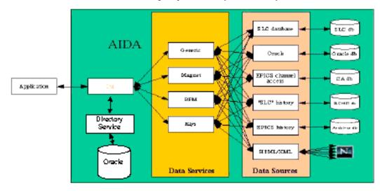
Figure 2: Logical Architecture, showing get/set/monitor, to/from any data source through a data service
