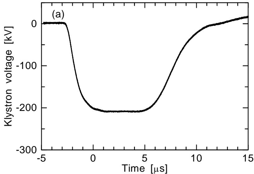
◆ For FEL experiments, stability of the pulse height and flatness of the Klystron voltage crucial.
