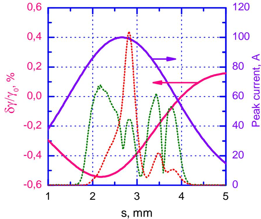
*Dotted curves illustrate the beam bunching (green) and radiation power (red) distributions*
