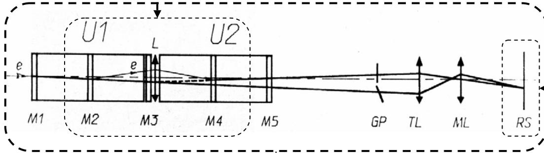
The scheme to observe radiation coherency at the achromatic bend of electrons in the magnetic system of the optical klystron on VEPP-3: M1-M5 – horizontal bending correctors; L – quadrupole lens focusing in horizontal direction; U1 and U2 undulators; TL and ML – optical telescope lens and imaging lens respectively; RS – registering screen
