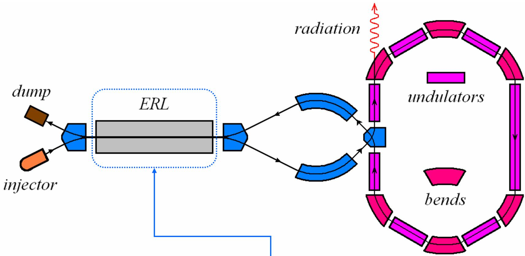
Ring FEL requires ERL as a source of electron beams, as the average beam power can be very high.
