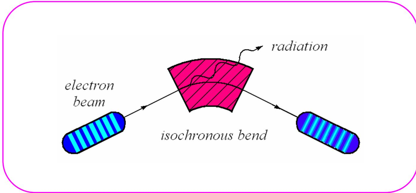
*The beam microbunching is partly conserved in the isochronous bend*
