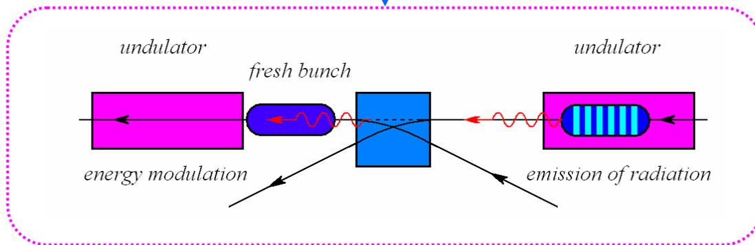
Signal from the old bunch to the fresh one is transferred by radiation
