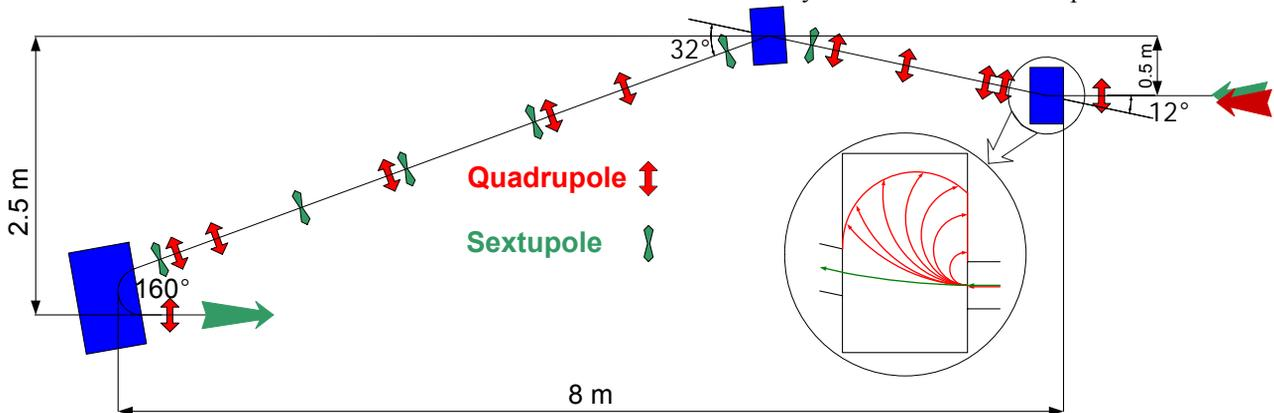
Figure 2. The layout of the first bent.
