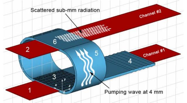
Fig. 3 Scheme of two-stage generation for the band of 0.2–0.5 mm: 1 — sheet REB for driving the planar FEM-oscillator; 2 — sheet REB for mm-wave scattering; 3 — 2D Bragg reflector; 4 — 1D Bragg reflector; 5 — special waveguide; 6 — area of 4-mm radiation scattering on e-beam.
