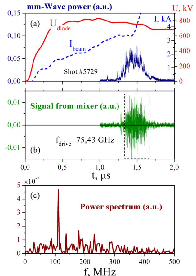
Fig.1 Single frequency operation of 4-mm FEM: a) diode voltage ( $U_{diode}$ ), beam current ( $I_{beam}$ ) and mm-wave power; b) intercarrier frequency signal from heterodyne mixer (heterodyne frequency  $f_{drive} = 75.43$  GHz); c) mm-wave power spectrum.
