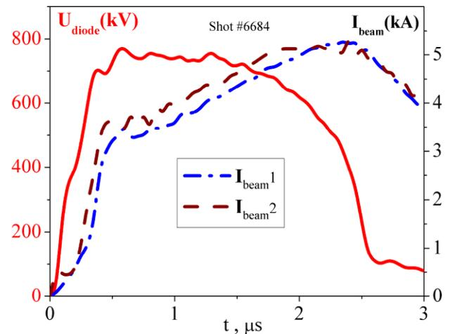
Fig. 6 Production of two sheet e-beams in a common diode with two cathodes and transportation of these beams through the parallel slit channels:  $U_{diode}$  — accelerating voltage;  $I_{beam1,2}$  — currents of the beams.
