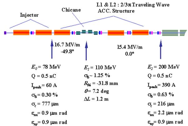
Figure 3: Layout of test machine for PAL XFEL
