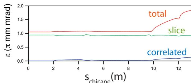
Figure 3: Evolution of the total, central slice and correlated emittance along the chicane at 110 MeV in the case of ARC-EN-CIEL phase 1. Charge 1 nC, energy 110 MeV, compression from 7 ps to 500 fs,  $R_{56} = 0.2 \text{ m}$ ,  $L_{chicane} = 10 \text{ m}$ .
