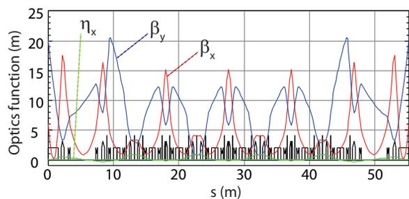
Figure 6: Optics functions versus the position along the arc at 1 GeV.  $\beta_x$ : vertical beta function,  $\beta_y$ : horizontal beta function,  $\eta_x$ : dispersion function.
