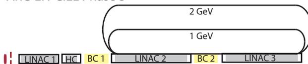
Figure 1: Representation of the ARC-EN-CIEL accelerator for the different phases. LINAC : Linear accelerator composed of cryomodules, HC : third harmonic cavity, BC : bunch compressor. To view all components, the representation is not scaled. Phase 1 is 70 m long, phase 2 : 200 m, phase 3 : 200 m with a radius of the arcs of 15 and 30 meters.
