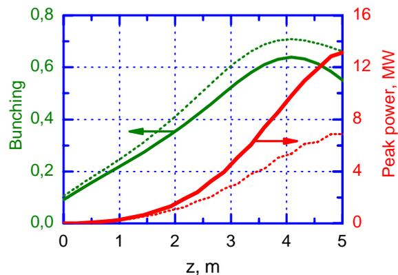
Figure 4. Dependence of the beam bunching factor (green) and peak radiation power (red) on the longitudinal coordinate in the last undulator section (dotted curves – CSR effects are not included).
