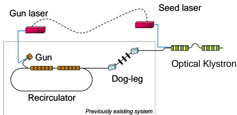
Fig 1. Overview of the accelerator systems and test FEL.
