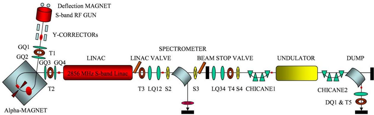
Figure 2: Layout of Mark III FEL Facility.
