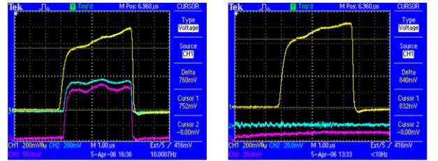
Figure 4: (left) signals of the first gun toroid (yellow), the second gun toroid (cyan), and linac toroid (magenta) when beam transmission from gun to linac and back bombardment along macropulse are optimized, (right) signal of the first gun toroid when there is no transmission in the  $\alpha$ -magnet. Here calibration factors for T1, T2, and T3 are 0.4 A/V, 0.4 A/V, and 1.0 A/V, respectively.
