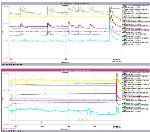
Figure 5: (top) spiky vacuum status on January 19, 2006 when gun generated 400 mA at T1 for the first time, (bottom) stabilized vacuum status on January 31, 2006 when gun generated 400 mA at T1 without any vacuum interlock for about 80 minutes.
