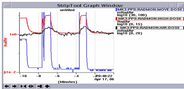
Figure 6: Signals of three radiation monitors along linac during 1 Hz and 10 Hz operations.
