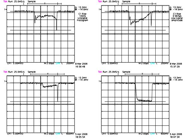
Figure 3: Signal of gun reflected RF power when reflected power are unbalanced at head and tail parts (top left), when head part has a high reflected power (top right), when reflected power is minimum and its slope along macropulse is optimized (bottom left), and signal of forward RF power when reflected power is optimized (bottom right).
