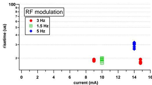
Figure 11: Efficiency of the Q-switch at different repetition rates using RF frequency modulation.
