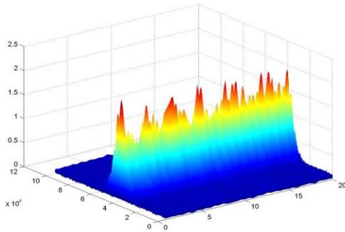
Figure 9: Sequence of 20 giant pulses, acquired by a fast photodiode, generated using the chopper Q-switch. The electron beam current is about 10 mA and the repetition rate is 1.5 Hz
