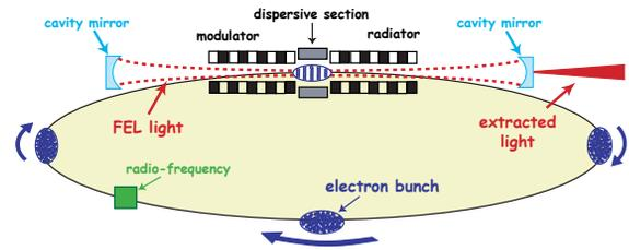
Figure 1: Layout of the Elettra storage-ring FEL in oscillator configuration.
