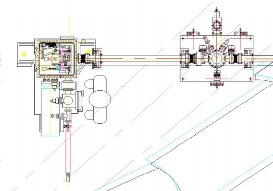
Figure 6: Schematic layout of the chopper chamber (at right), near the mirror chamber (at left).
