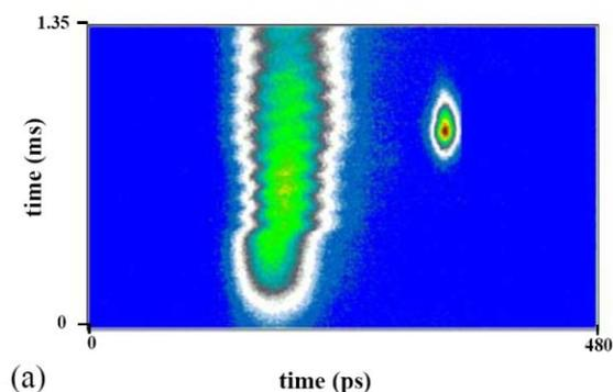
Figure 3: Streak-camera image of the electron beam (left trace) and of the FEL pulse (right trace) in Q-switch operation mode.
