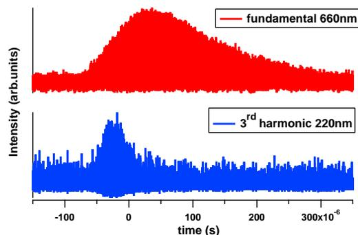
Figure 2: The fundamental (660 nm) and the third harmonic (220 nm) giant pulses. The harmonic signal is about a factor 25 above spontaneous emission.
