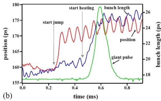
Figure 4: Analysis of the streak camera image in Figure 3. The longitudinal distributions are obtained by means of a horizontal cut of the picture.
