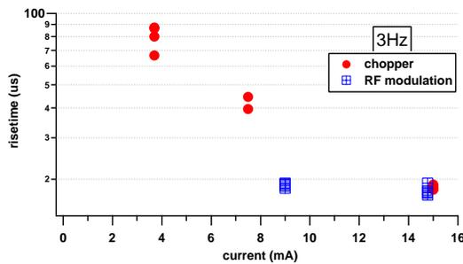
Figure 10: Comparison between chopper and RF modulation techniques, showing the risetime as a function of the total current at the same operational frequency (3Hz).
