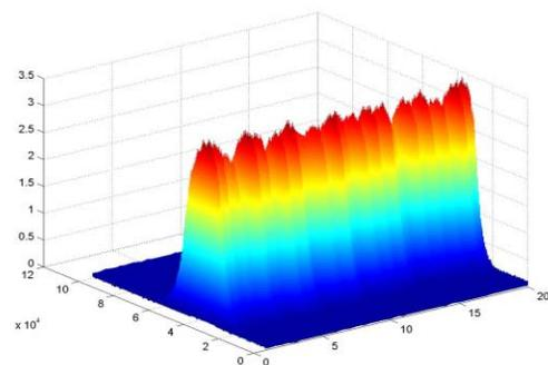
Figure 8: Sequence of 20 giant pulses, acquired by a fast photodiode, generated using the RF modulation. The electron beam current is about 10 mA and the repetition rate is 1.5 Hz
