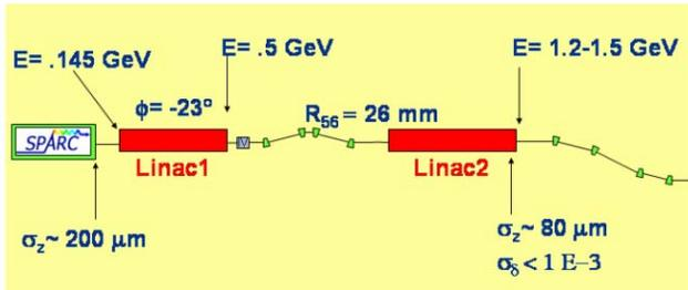
Figure 5: Schematic layout of the RF+magnetic compression scheme.
