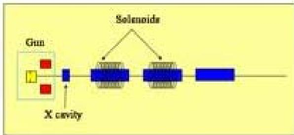
Figure 2: Schematic layout of the SPARXINO photoinjector.
