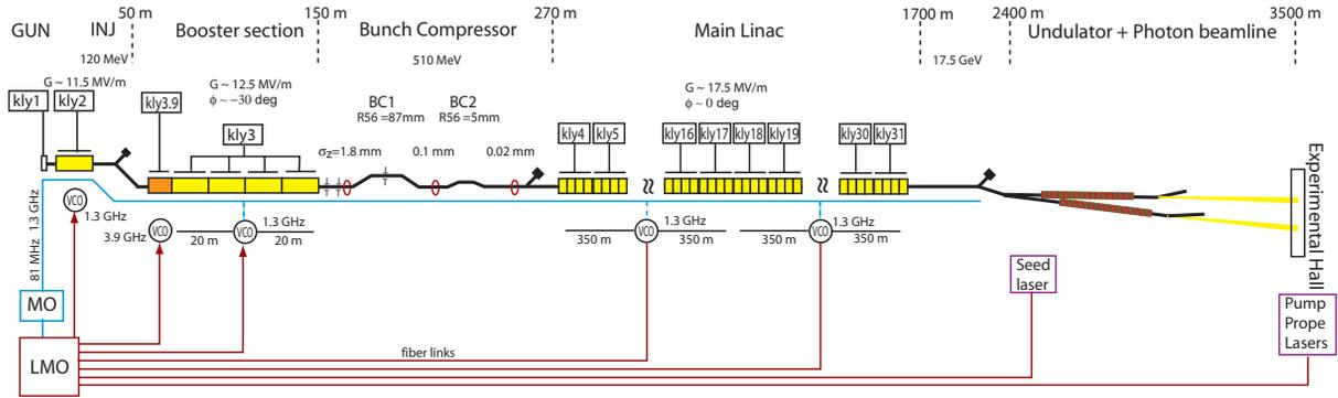
Figure 2: Layout of a 4th generation light source.
