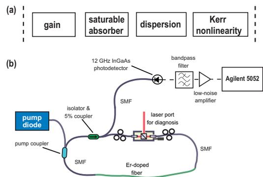
Figure 3: (a) The four effects governing pulse shaping in mode-locked lasers. (b) Schematic of the experimental setup: SMF, single-mode fiber.
