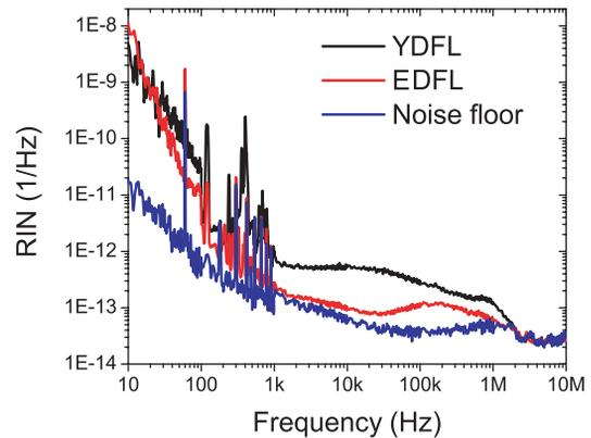
Figure 4: Relative intensity noise (RIN) of the EDFL and YDF, along with the measurement noise floor.
