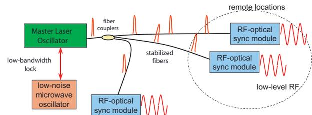
Figure 1: Schematic of the optical timing synchronization system.
