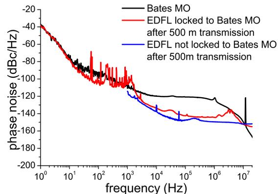
Figure 8: Single sideband phase noise of the Bates Reference Oscillator, the EDFL locked to the reference after transmission through the link and the free running EDFL.
