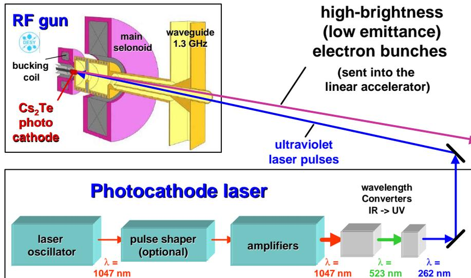
Figure 1: General setup of a photoinjector
