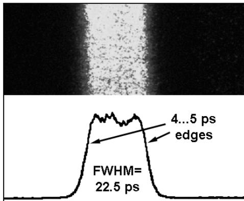
Figure 4: Streak camera record of the pulse shape at the Nd:YLF drive laser in use at PITZ
