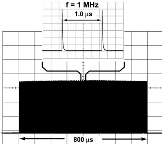
Figure 3: Output pulse train of the Nd:YLF drive laser
