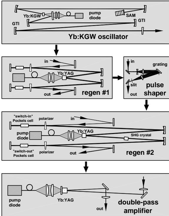
Figure 5: Scheme of the experimental Yb:YAG laser-driver laser under development at the MBI
