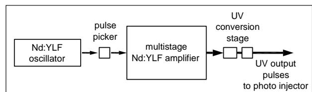
Figure 2: Basic scheme of the Nd:YLF photoinjector drive laser used at FLASH and PITZ
