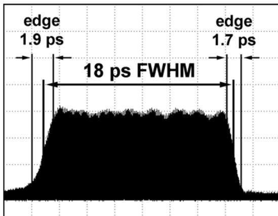
Figure 6: Cross correlation signal showing the flat-top pulse shape of the experimental Yb:YAG laser
