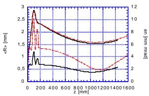
Figure 1: Envelope and rms normalized emittance and as computed by ITACA (solid line) and HOMDYN (dashed line). Thermal emittance set to zero.
