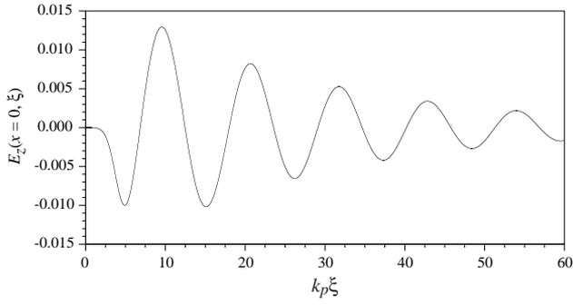
Figure 2: Longitudinal wake field on axis for a channel with  $k_p b = 2$ ,  $\alpha = 17^\circ$ ,  $\omega_{p0} \xi_c = 4$ , and  $\omega_{p0} w_\xi = 1.5$ .
