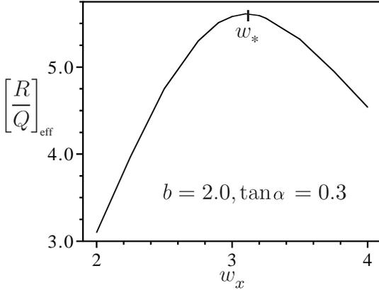
Figure 3: Effect of transverse driver width upon  $[R/Q]_{\text{eff}}$ . The optimal value of  $w_x$  is denoted by  $w_*$ .
