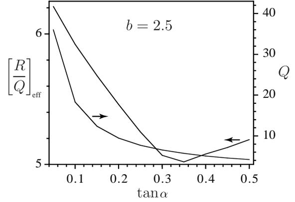
Figure 4: The effect of the wall inclination on  $Q$  and  $[R/Q]_{\text{eff}}$  with optimal driver width.
