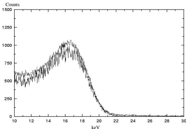
Figure 4:  $\gamma$ -spectroscopy of both RFQ's at 120 MHz and 5 kW
