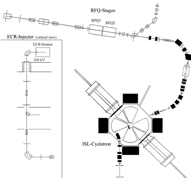
Figure 1: Scheme of the beamline
