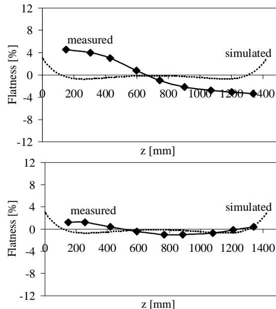
Figure 2: Measured and simulated flatness of RFQ1 (upper) and RFQ2 (lower).
