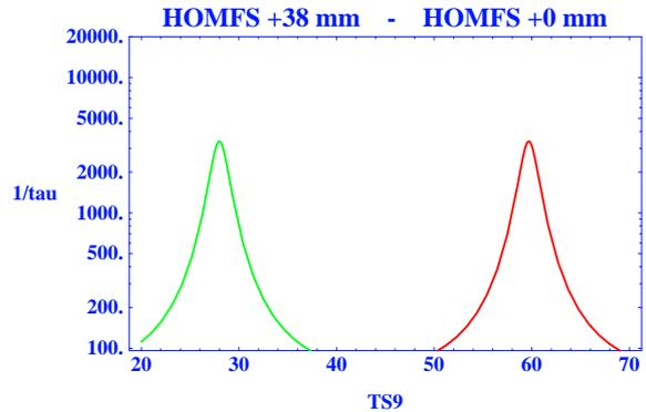
Fig. 5: Effect of the HOMFS on the dipole HOM T3
