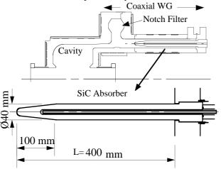
Figure 1: A schematic drawing of the accelerating cavity of the ARES cavity with the SiC absorber.
