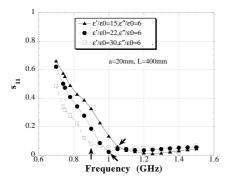
Figure 3: S<sub>11</sub> frequency response of the SiC absorbers with different permittivities.
