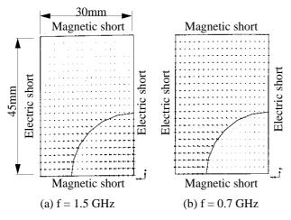
Figure 5: Electric field of the propagating mode in the 2-dimensional lossless model. (a=20mm,  $\varepsilon_r$ '=22).
