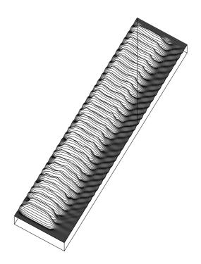
Figure 6: Wake field excited by a charge with rectangular density in x-direction, total width 1 cm
