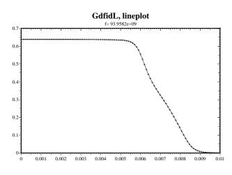
Figure 3: Longitudinal electric field over cavity width
