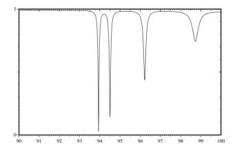
Figure 4: Reflection coefficient versus excitation frequency in GHz
