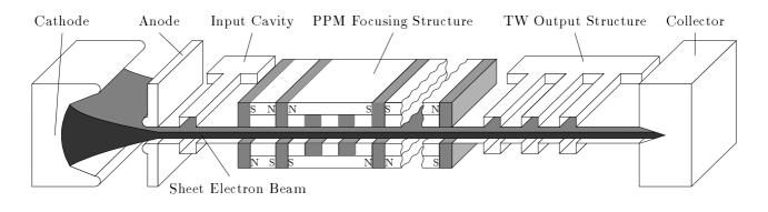
Figure 1: Schematic of the sheet beam klystron
