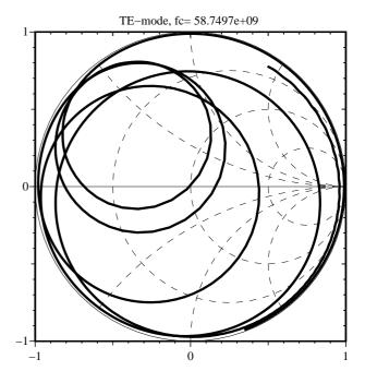
Figure 5: Smith chart of reflection coefficient
