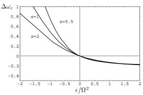
Figure 3: Coherent frequency of bunch shape oscillalations  $\Delta\omega_c = (\omega_c - 2\omega_{s0})/\omega_{s0}$  as a function of intensity parameter  $\epsilon/\Omega^2$  for different values of RF voltage (s).
