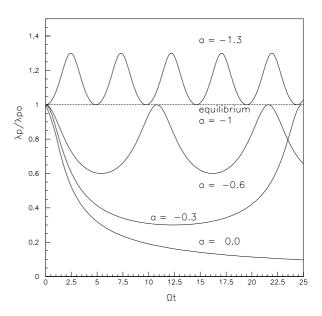
Figure 2: Variation of normalised peak line density 1/r for different types of induced voltage with RF off (s = 0).
