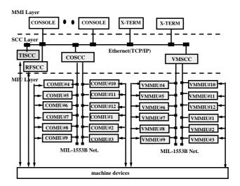
Figure 1: Computer Control System Structure.
