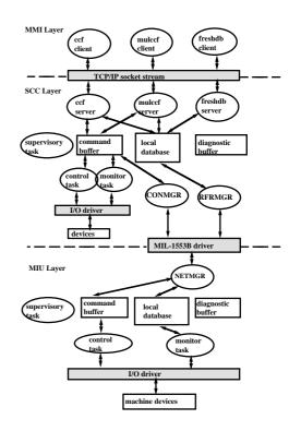
Figure 2: The Software Structure of the Data Acquisition System.
