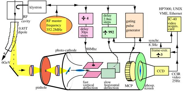
Figure: 1 Synchronisation of the Streak Camera system
