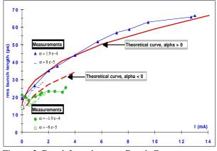
Figure: 2 Bunch Length versus Bunch Current
