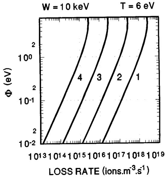
Figure 4: Beam potential  $\Phi$  as a function of loss rate of protons for four different pressures  $p$  into the beam chamber (1:  $p = 10^{-1}$  Pa, 2:  $p = 10^{-2}$  Pa, 3:  $p = 10^{-3}$  Pa and 4:  $p = 10^{-4}$  Pa) at the electron temperature  $T = 6$  eV and at the energy of protons  $W = 10$  keV.
