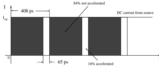
Figure 1: The transmission of the d.c. source current through the accelerator. At best 16% of the generated electrons reach the experiment.
