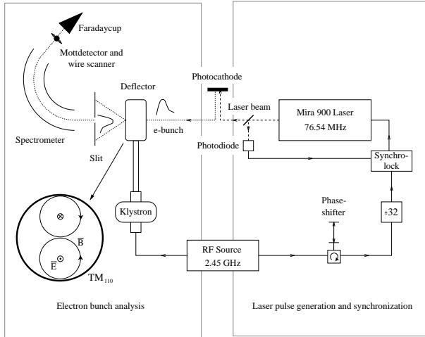
Figure 3: Principle of the measurement is a radiofrequency streak method. On the right side the laser pulse generation and synchronization to the MAMI rf is shown. The left part of the sketch shows the electron bunch analysis with the  $\text{TM}_{110}$  deflector cavity.
