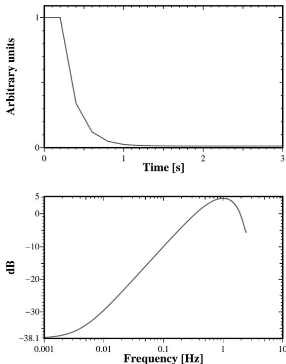
Figure 2: Plots of simulations: 1.) Response on a step disturbance on incoming beam; 2.) Disturbance transfer function of a feedback loop, Nyquist frequency at 2.5 Hz,  $f_c = 0.005$  Hz.
