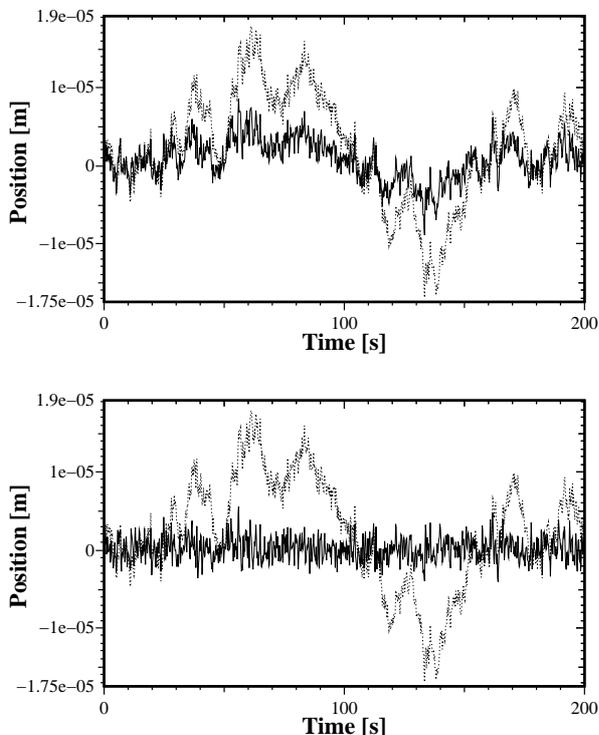
Figure 1: Plots of simulations: Controlled (solid) and uncontrolled (dashed) beam motion for  $f_c = 0.05$  Hz (upper plot) and  $f_c = 0.005$  Hz (lower plot) in the sampling time scale.
