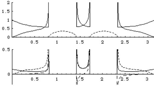
Figure 4: (Top) Emittances and growthrate-1 (dashed line), (bottom)  $\Sigma_{11}$  (solid line),  $\Sigma_{13}$  (dashed line),  $\Sigma_{33}$  (dotted line), as functions of  $\Phi$  for  $(\nu_x, \nu_y) = (0.2, 0.15)$  and  $(\beta_x, \beta_y) = (0.33, 0.01)\text{m}$ . All are normalized by  $\epsilon_0$ .
