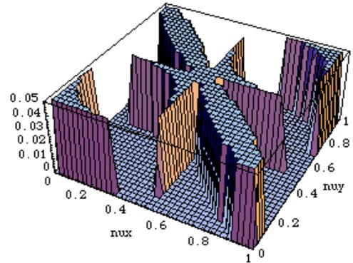
Figure 3: The unstable region in  $(\nu_x, \nu_y)$  plane. Parameters:  $\Phi = 0.02 \times 2\pi$ ,  $(\beta_x, \beta_y) = (0.33, 0.01)\text{m}$ . The vertical axis gives the growthrate-1.
