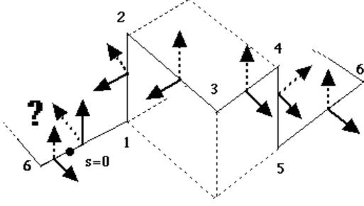
Figure 1: The parallel transport and the twist. The starting point  $s = 0$  is indicated by  $\bullet$ . The magnets are numbered. The magnet number 6 represents a long planar arc. The  $\mathbf{e}_x(0)$  (dotted arrow) and  $\mathbf{e}_y(0)$  (solid arrow) are defined arbitrarily at  $s = 0$  and they are transported parallelly along the reference orbit. After they come back to  $s = 0$ , they notice that they are tilted by an angle  $\Phi$  ( $\pi/2$  in this example).
