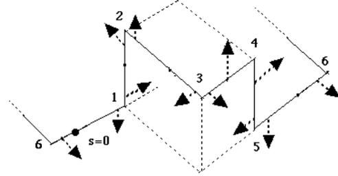
Figure 5: The  $x$  coordinates (arrows) according to the Frenet-Serret triad for the same example of Fig.1.
