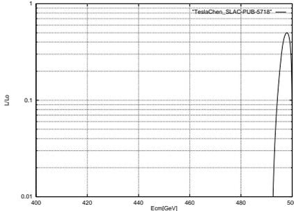
Figure 2: Luminosity spectrum  $\frac{\mathcal{L}}{\mathcal{L}_0} = f(E_{cm})$  for LC design TESLA taken out of [CHE92]
