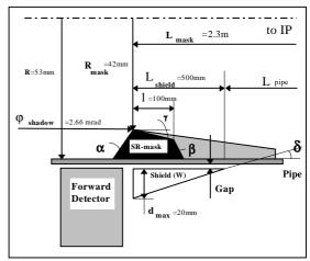
Figure 1: Specified Mask and Shield Dimensions
