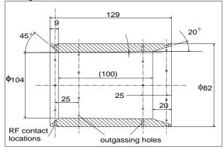
Figure 4: Section through ALEPH Mask
