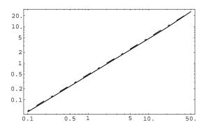
Figure 1: Dependence of the tune split  $|Q_I - Q_{II}|$  on  $a_2$  expressed in units of nominal  $a_2$
