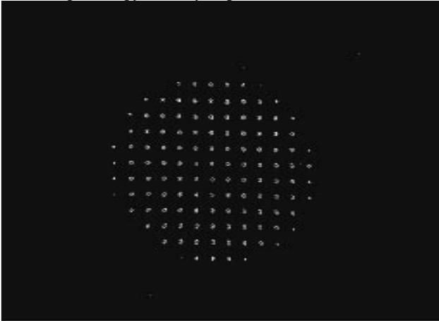
*Figure 1: PPM image of a 500 keV, 3 mA proton beam on a P46 phosphor screen.*
