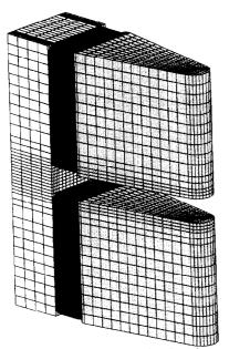
Figure 3: TOSCA model for the S-coil sector magnet.
