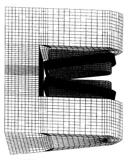
Figure 2: TOSCA model for the tilted coil sector magnet.
