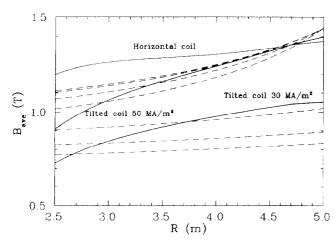
Figure 1: Average field for several different isochronous fields (dashed lines) ranging from Q/A=0.5 and E/A=496 MeV/A to Q/A=0.35 and E/A=98 MeV/u. The solid line on top shows the average field obtained in the TOSCA model with horizontal coils parallel to the median plane. The thicker solid lines show the average field for the tilted coil model at two different excitations.
