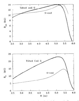
Figure 4: Average field (top) and sixth harmonic (bottom) for the tilted coil model and for the S-coil model.
