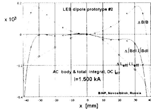
Figure 3. End field correction on dipole prototype #2.
