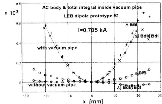
Figure 5. Maximum distortion of the field in dipole #2 by vacuum pipe (stainless steel, 1 mm thick,  $d \approx 60$  mm) at AC.
