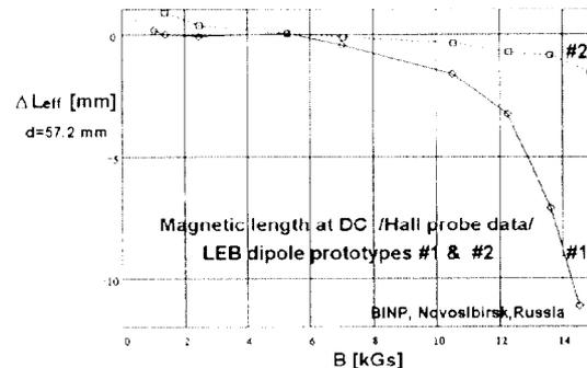
Figure 4.  $\Delta L_{eff}(l)$  in dipole prototypes #1 and #2.
