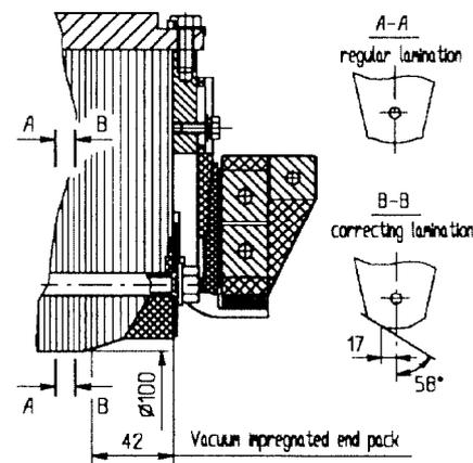
Figure 2. End pack of quad prototype #2.
