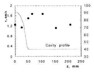
Fig. 2 Sputtering rate distribution along a meridian.
