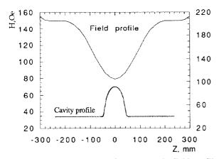
Fig. 1 Parallel component of the magnetic field profile along the cavity axis for the post-magnetron we built.
