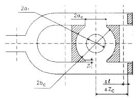
Figure 1: Symmetrical coupler with two waveguides and power devider
