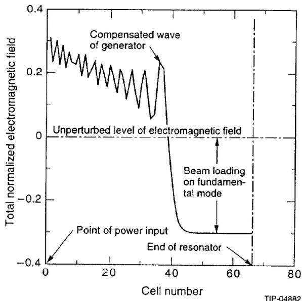
Figure 3: The perturbed electromagnetic field in cavity (calculation)
